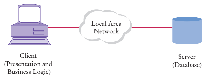
Figure 10 Two-Tier Client-Server Architecture
